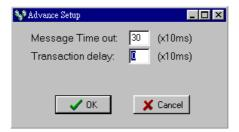
**Message Time Out**: The time-out time for PLC, the default setting is 300ms. Ethernet module will wait for the same amount time of this field before the PLC can reply the command message.
