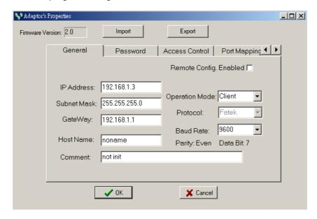
It has an additional 'Port Mapping' tab when compare with server mode, after click the 'Port Mapping' tab the screen changes to
