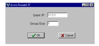
With this dialog to define a set of consecutive authorized IP addresses. Please input the first IP address of the consecutive IP addresses in the 'Grant IP' field and input the size of IP addresses in 'Group Size' filed.
