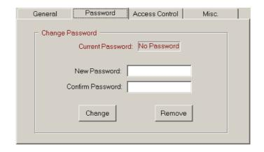
Please input the new password at 'New Password' and 'Confirm Password' edit field and click the 'Change' button to complete the setting of new password. Please click the 'Remove' button if password protection is not necessary.
