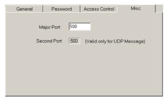
The Ethernet module when work either in TCP or UDP server mode should be assigned a service port number for client access. The default port number for FBs series Ethernet module is port 500. If the user want to change the port number can click the 'MISC' tab and change the Major port field to desire port number. Second port field provides the UDP working mode the opportunity to have dual service port number, one is port 500 the other is port number appear in Major port field.
