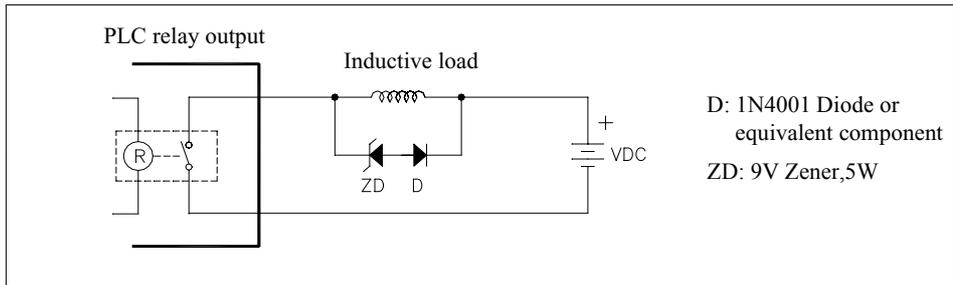
Diode + Zener suppression of DC load (use in larger power and frequent ON/OFF)
