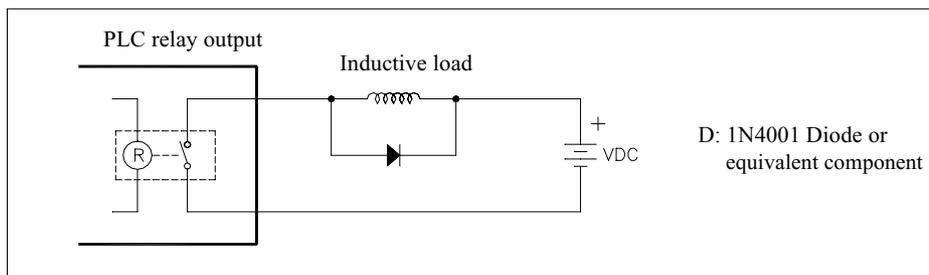
Diode suppression of DC load (use in smaller power)
