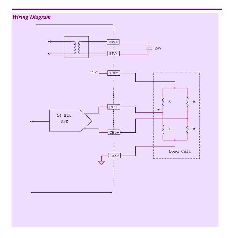
The conversion result is represented by a 16 bit signed value, there should put an additional LCNV (FCN33)or MLC(FCN34)function instruction in the ladder diagram, which will convert the raw reading value into the desire weight value. Because the measurement signal is quite small, for common practice, manual zero adjustment is required in order to overcome the null drift.
