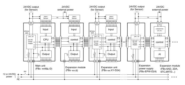
Note \*<sup>2</sup> : The 5VDC power of 10/14PTs main unit is generated by the oscillations of the 24VDC power in the output circuit, with specifications of 5VDC±10% and 400mA (max) (Circuit is located on the I/O board of 10/14PTs main unit)
