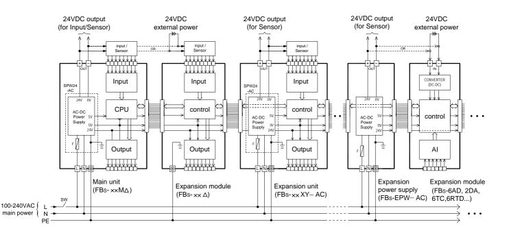
5.2 Specifications and Wiring of DC Power Sourced Power Supply
