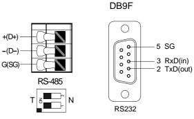
Pin assignment of the connector
