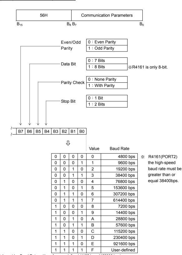
Setup of port0~port4 communication parameters
