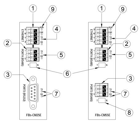
① Ethernet connector : Instead of traditional RJ-45, European 4pin connector with excellent contact is used for the vibration environment of the machine.
