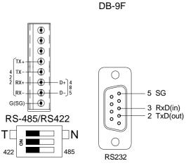
Pin assignment of the connector
