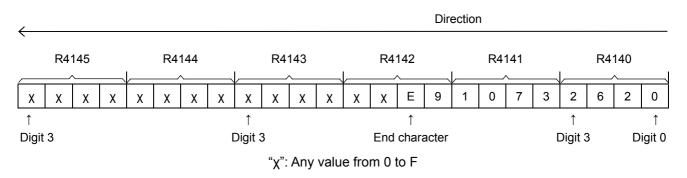
2620H is stored in R4140, 1073H is stored in R4141,and XXE9H is stored in R4142. R4143~R4145 can be any value. Please note that the last digit of the phone number must be followed by the end character "E". The PLC host will ignore the number (any value from 0 to F) behind "E". Only the value 0~C is acceptable before "E". Any other values will be regarded as ineffective.
