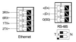
Pin assignment of the connector
