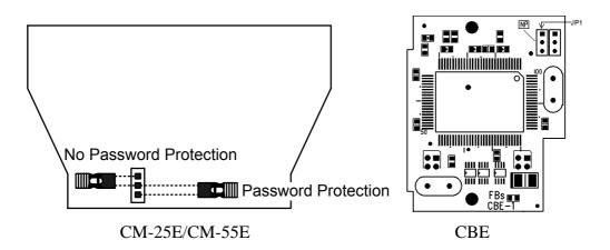
When CM-25E, CM-55E or CBE the jumper cap of JP1 is at upper position (linked by white line), the password protection is disabled. The jumper cap should put in the lower position when under normal operation.
