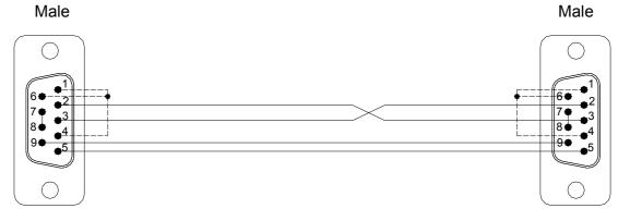
If you make RS232 cables by yourself and the definition of each pin is not clear, use a multimeter for measurement to determine TXD and RXD.
