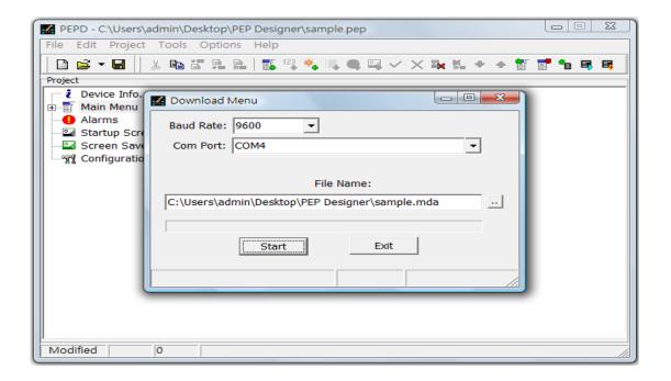
After setup the "Baud Rate" and "Com Port" settings and select the file name, press the button to download design to PEP for real operations.
