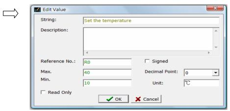
**%** In this example, "R0" is the reference number corresponding to the PLC, i.e. the register assigned to save the value for Set the Temperature. The Maximum and Minimum values are 40 and 10 respectively. The temperature unit is °C.
