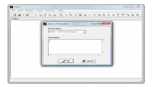
\*\* You can add description to this program in the Description field. Otherwise, press the ock button and the project tree nodes in the red frame below will be generated automatically. These include the Device Info, Main menu, Alarms, Startup Screen, Screen Saver and Configuration menus. Now, you can begin planning and setting up the project contents.
