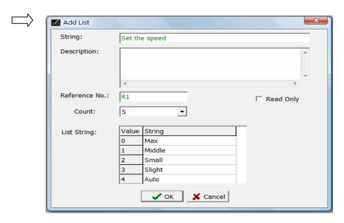
**%** In this example, "R1" is the reference number corresponding to the PLC, i.e. the register assigned to save the value for Speed. If the choice is "Small", the value 2 will be written to the R1 register of PLC.
