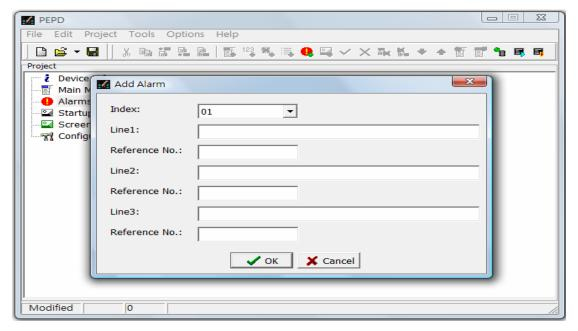
\*\* Index: Users can set any number from 01-64. When the value in the Alarm Source Register in Configuration is identical with the Alarm No., the alarm message of the corresponding Index will be activated. Therefore, the maximum number of alarms is 64.
