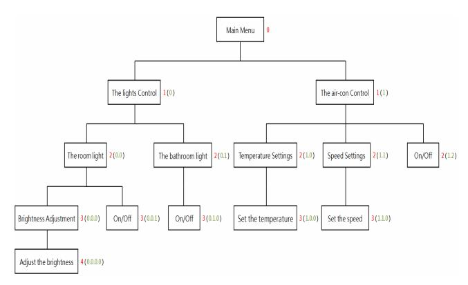
**\*\*** There is a set of numbers inside parentheses next to each item. The sequence of these numbers is 0, 1, 2, 3 and so on. The number on the leftmost indicates the level to facilitate users to plan a project and will not be displayed in PEP. The numbers within the parentheses, represent the level and item locations of the menu as shown below.
