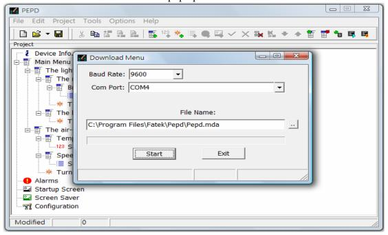
**Step 3:** After setting the Baud Rate and Port and the compiled design filename, press the button to download design to PEP device as shown below.
