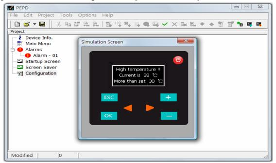
**X** You can also check the alarm configuration with [Off-line Simulation]. When an alarm is set, the icon will appear on the [Off-line Simulation] screen. Click the icon to select the "Index" for running "Alarm Trigger" as shown below.
