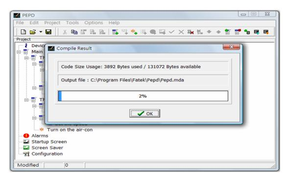
Step 3: After verify the compile result is OK, press the button and the Setup Port Parameter window will pop up as shown below.
