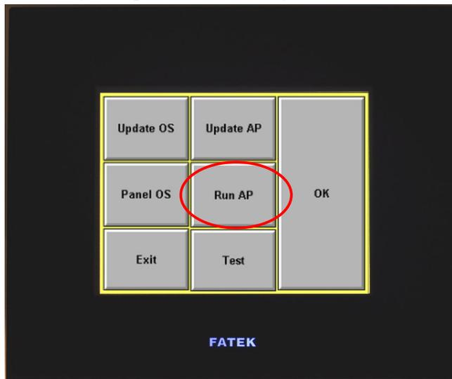
To operate in the Panel Setup Screen of FV035ST-C10, one can quickly press the corners on the Touch Panel following the order of upper left, upper right, and upper left. The system will automatically switch to Panel Setup Screen and allows the user to modify the parameters in the system menu.
