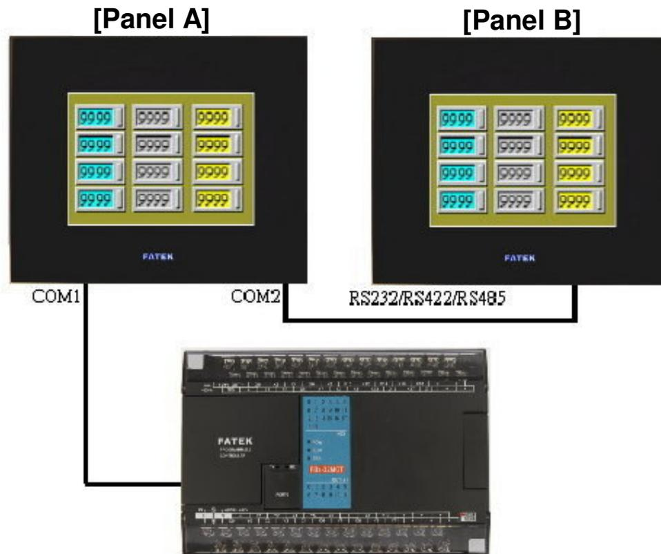
Note: When using this function, the operation management of the two FV HMIs must be located in the same file (AP) so that the options shown in the figure will be available to be selected.
