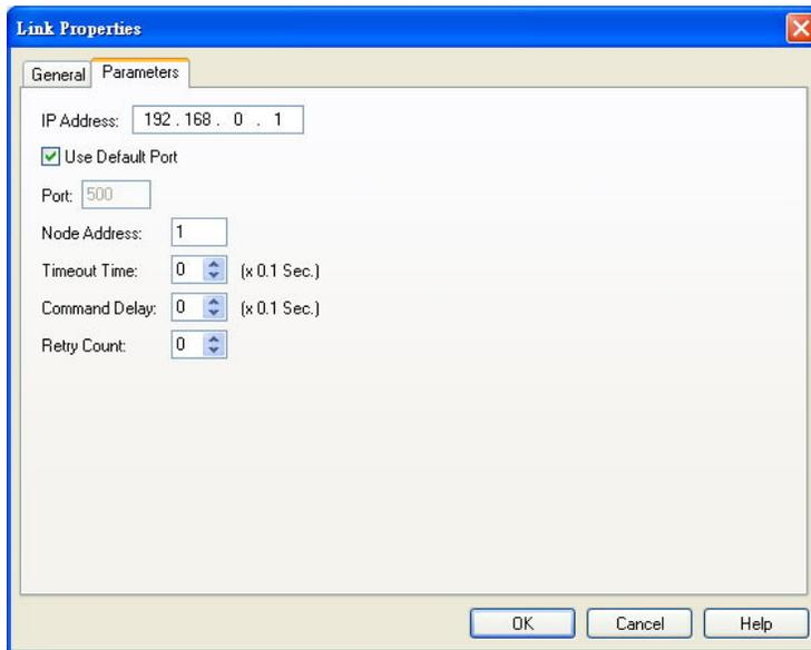
IP Address: Define the IP address same as the controller. In this example, the IP address of Link 1 is 192.168.0.1 and Link 2 is 192.168.0.2.
