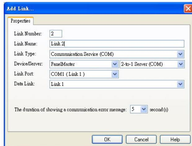
3. New link must be added to FV HMI with communication service selected (Ethernet or COM port).
