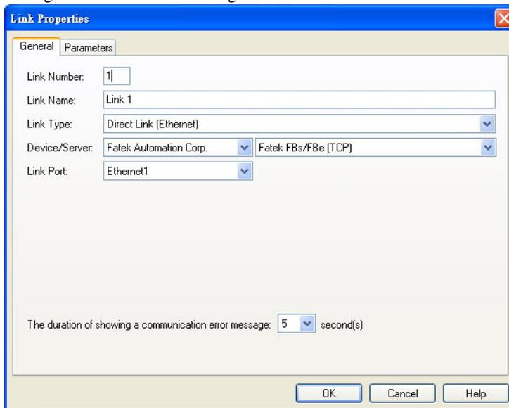
Link Number: defined by the system. This example has two PLC links, so two link numbers, 1 and 2, are defined by the system.
