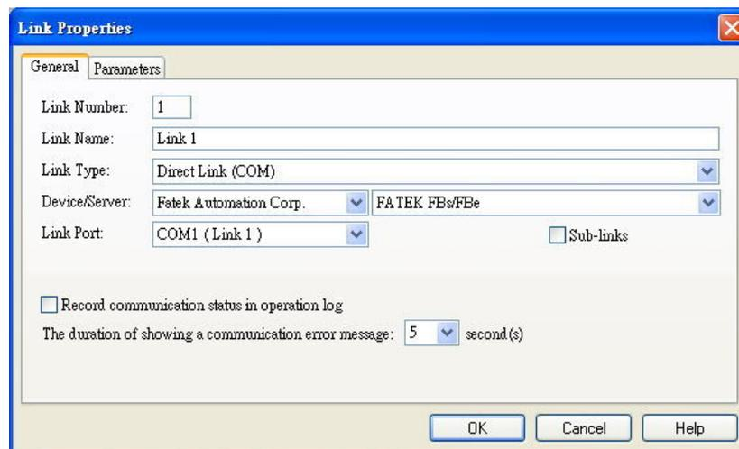
4. The Device/Server for Link 2 in FV HMI must be the same as that for Link 1 in data link.
