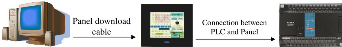
**Note:** Prior to setting up transparent communication, an FV HMI program corresponding to the program in the PLC currently used needs to be downloaded into FV HMI.
