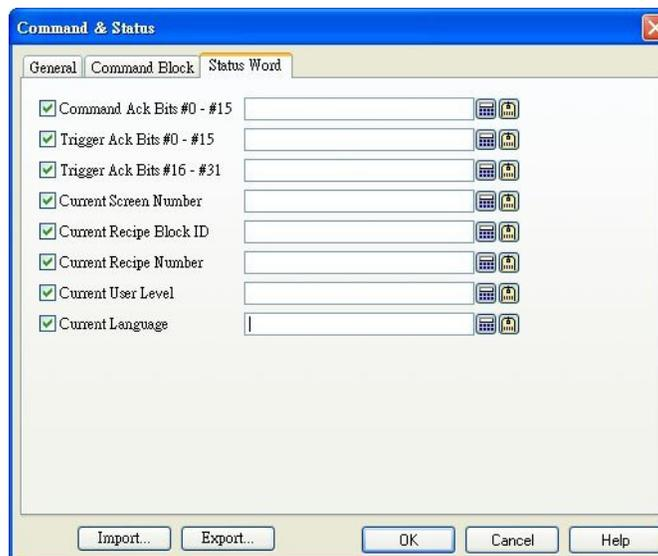
Check the corresponding options to set the addresses. The address can be the internal register of PLC or the internal address of FV HMI. If the Current Screen Number is selected and the address is set to D100, the Current Screen Number will be sent to D100 after FV HMI completes screen switching.
