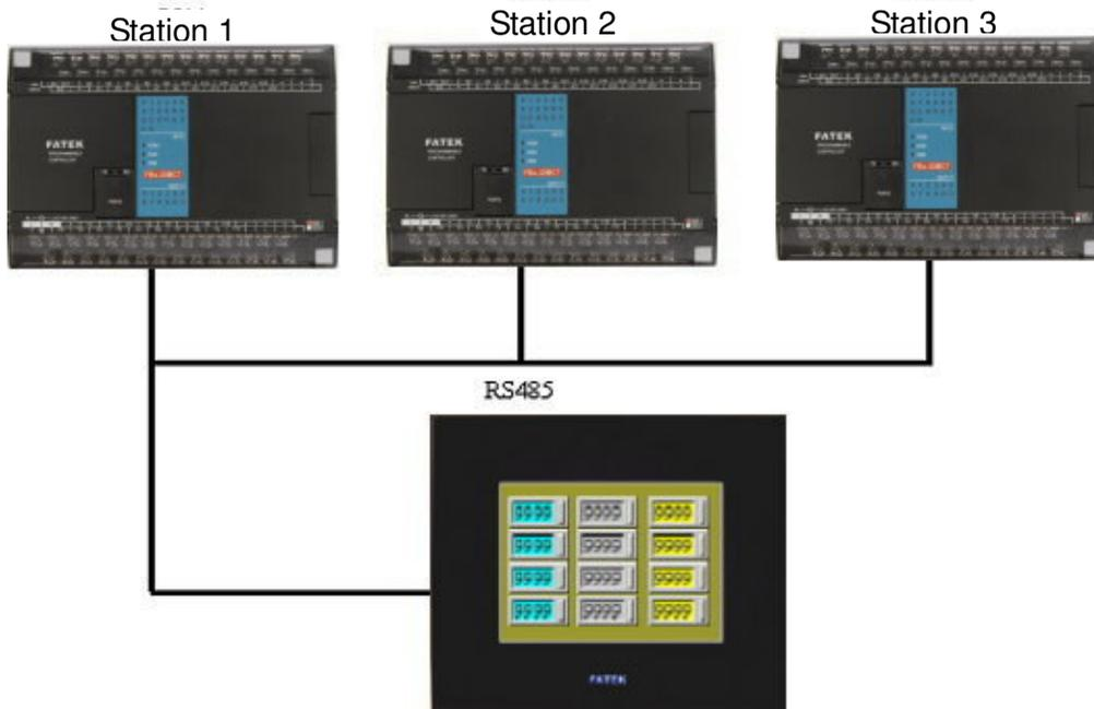
For example, to write the first 10 words in the R0 register of Station 3 to R100 in Station 2, the program for the corresponding macro command can be written as follows; it can be located to be used when needed (please refer to the introductions of macro commands for details).
