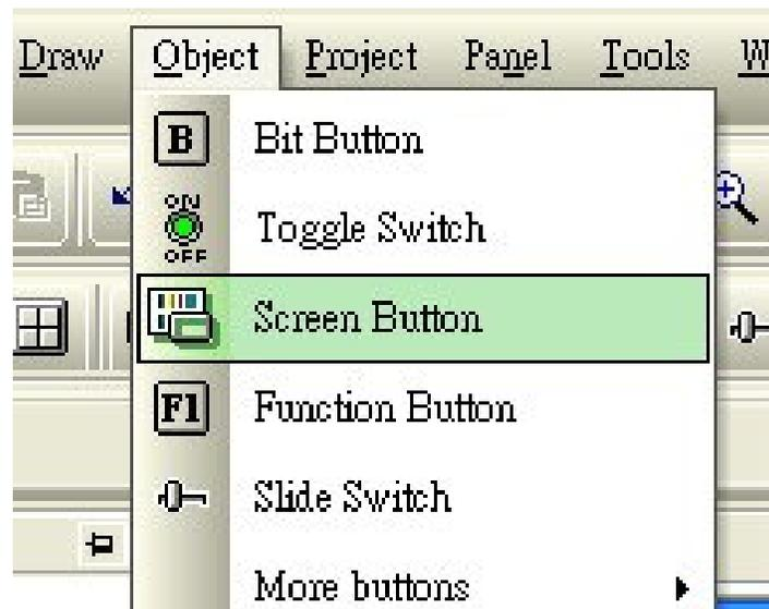
Move the mouse to the Screen Edit Area and click the left button once to place the Screen Button at the desired position in the area. Double click the left button to open the Device Properties Dialog box, as shown by the figure
