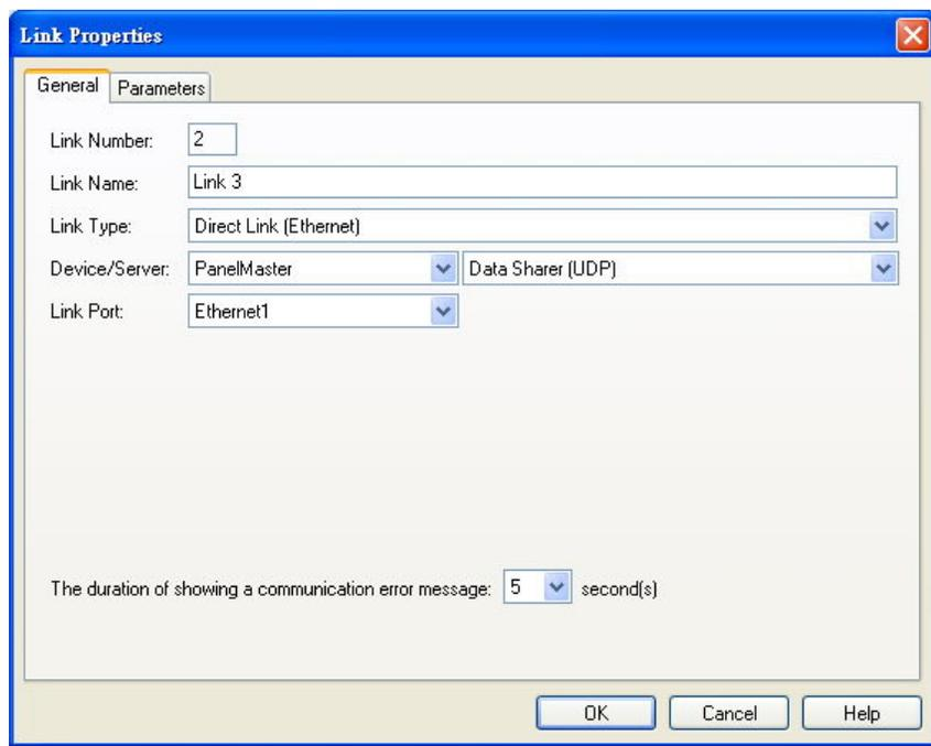
For Data Sharer(UDP), the fast share for Ethernet provided by PM Designer, the data format is Pm.n, where m is the station number with up to 16 stations (1~16) and n is the Word address with up to 128 words (0~127).
