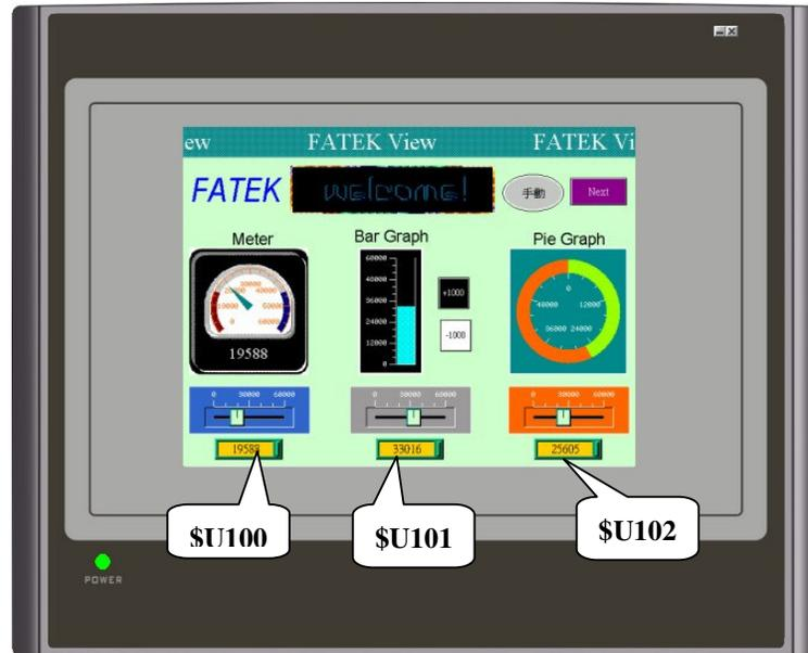
At this moment, one can directly click the device on the screen to exchange data with PLC, the effect of which is the same as that in the case of actually connecting to FV HMI. To exit online simulation, click the
