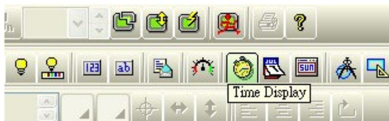
It can also be done by selecting [Object] in Toolbar ⇒ direct to [Time/Date] ⇒ click [Time Display] as shown in the figure below:
