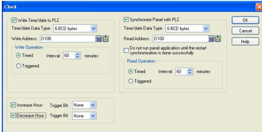
**Write Time/date/ to PLC:** Send the clock data of Fv HMI to the designated PLC address.
