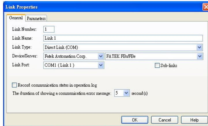
2. A new link must be added to FV HMI with communication service selected (Ethernet or COM port), and named Link 2. Set the data link to Link 1.
