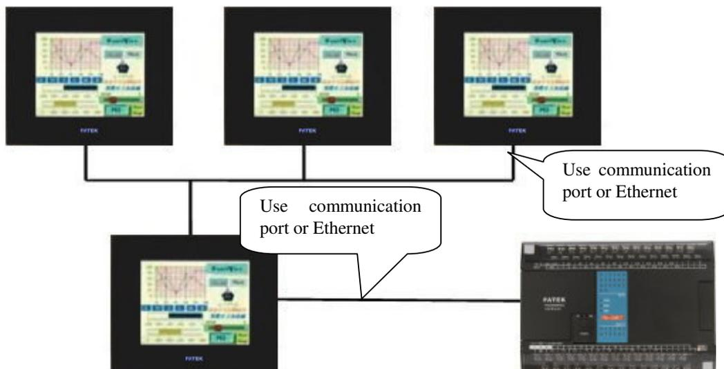
In addition to be able to communicate individually with PLC, FV HMI can communicate with other FV HMIs, which is realized by using various ports (RS-232, 422, and 485) or Ethernet.
