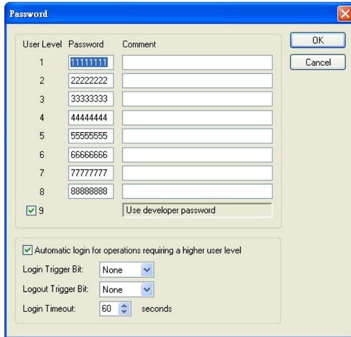
**Note:** this FV HMI supports any password with the length of 1-8 bits.
