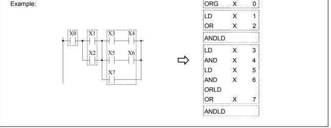
• The output coil instruction (OUT) can only be located at end of the network (the right end) and no other elements can be connected to it afterwards. The output coil can not connect to the origin line directly. If you want to connect the output coil to the origin line, connect it serially with a short circuit contact.
