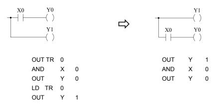
• The diagram shown below indicates the TR relay and the ORLD instruction can be omitted.
