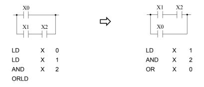
• When a single element or a serial block is connected in parallel with a parallel block, ANDLD instruction can be omitted if put the parallel block in front.
