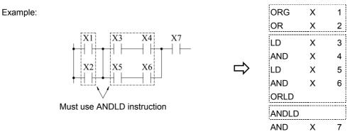
• The ANDLD instruction must be used if the element or serial block is in front of the parallel block. If the parallel block is in front of the element or serial block, AND instruction can be used to connect all parts together.
