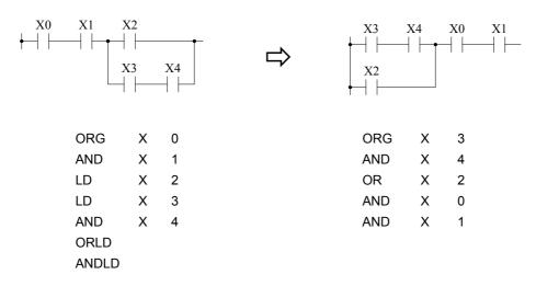
• If the branch node of a branch circuit is directly connected to the output coil, this coil could be located on top of the branch line (first row) to reduce the code.
