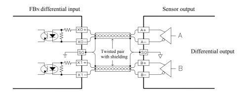
(B) Method of converting DC5V differential input to DC24V single ended SINK input
