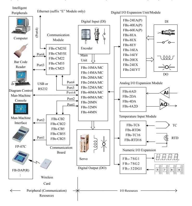
For the I/O of FBs-PLC, it can achieve a maximum of 256 point digital input (DI), 256 point digital output (DO), 64 word numeric input (NI), and 64 word numeric output (NO). Combined with various special interface modules, it can directly connect with devices such as Thermocouple, RTD, 7-segment LED display, and the Thumbwheel switch, which are shown on the right in the above figure.
