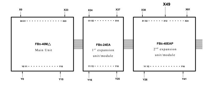
As shown in the above figure, because the top X numbers of the previous two units are 23 and 14, respectively, the number of input contact X12 on second expansion unit should be:
