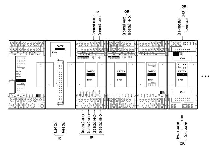
During the startup stage, FBs-PLC will automatically detect the types and CH numbers of expansion units/modules. While operation, the FBs-PLC will read the CH input values from the NI module and stores them into corresponding IR(R3804  $\sim$  R3903) and outputs OR values (R3904 $\sim$ R3967) to channels on the NO module. No pre-configuration or setting by users is required.
