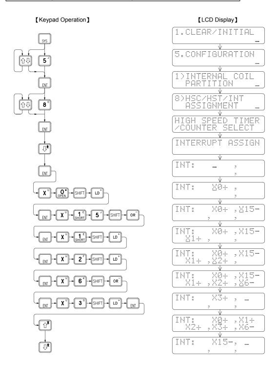
• External interrupt shares the 16 high-speed input points, X0~X15, with HSC and SPD instructions. Therefore, the number of the input points used by HSC or SPD cannot configure for external interrupt.
