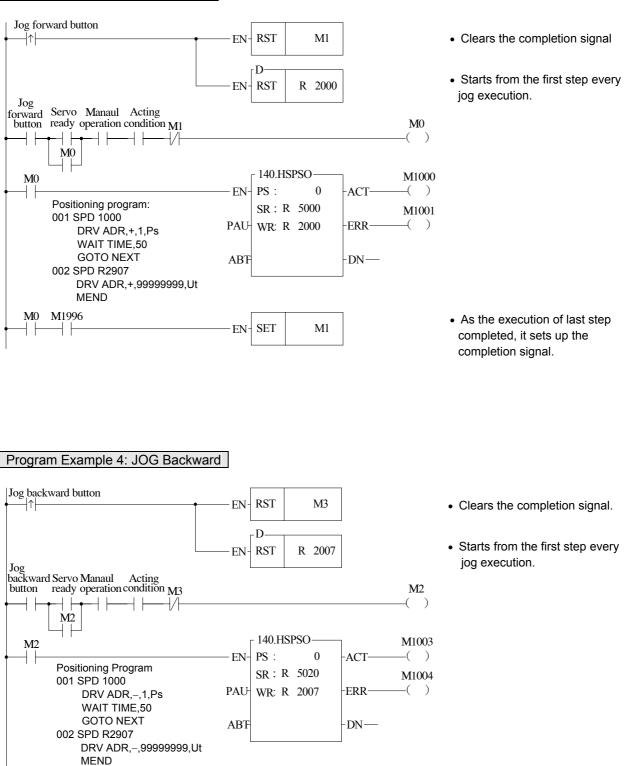
As the execution of the last step completed, it sets up the completion signal.
