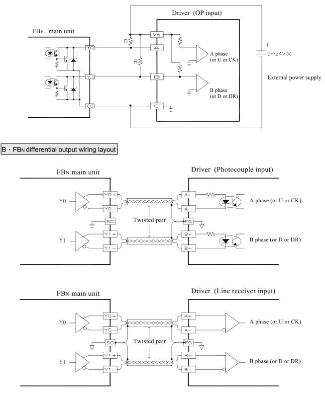
(For line receiver input, it must make PLC connect to FG of driver to eliminate common mode voltage)
