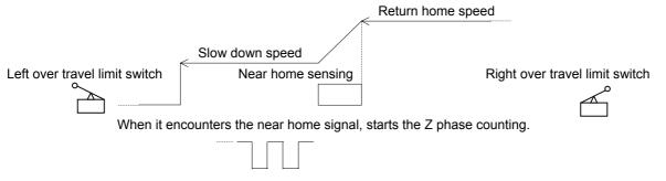
Z phase counting is up, the pulse output stops, then send out the CLR signal to clear the error counter of servo driver.
