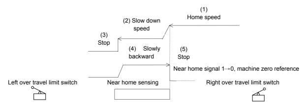
X3: Near home sensing input; it is configured as falling edge interrupt input.
