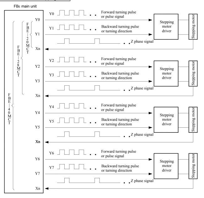
• Stepping motor is designed to receive input pulse to attain to the control of desired angle or distance, therefore the turning angle and the input pulse count has a positive correlation ship, and the turning speed also depends on the input pulse frequency.
