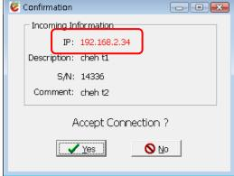
When the connection request window appears, the maintenance personnel can press the Yes button to accept this connection or press the No button to reject this connection.
