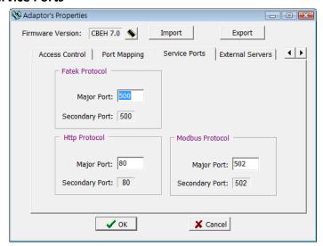
When the CBEH expansion board is working under TCP or UDP server mode, the external service ports must be set so that the external client workstations can send service requests according to the set service port numbers.
