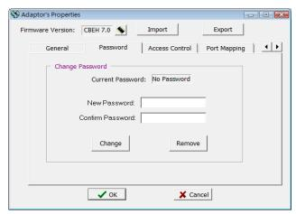
Just enter the password you want to use in the New Password and Confirm Password fields, and then press the Change button to complete the setting. To cancel the password, just press the Remote button.
