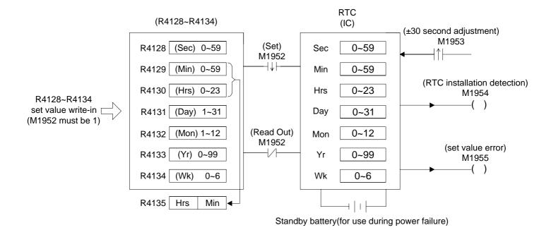
%D4053= 0 , no RTC chip installed = 1 , RTC chip is HT1381 = 2 , RTC chip is ISL1208 = 3 , RTC chip is S35390A
