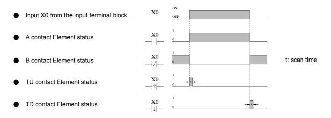
The waveform shown above reveals the function of A, B, TU and TD elements by exercising the external input X0 form OFF to ON then OFF.
