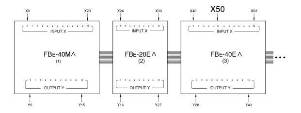
• The input number of any point on an expansion unit/module is the number of the point added with the total number of inputs preceding of it. The same is true for output number calculation.
