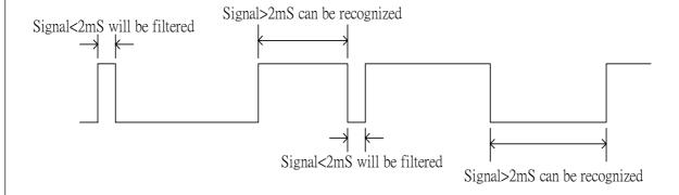
Example 2: When the filtering frequency is 28KHz, if the input frequency is greater than 28KHz, it will lose the input signal.
