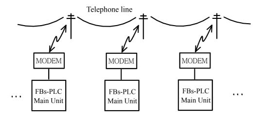
Besides the above area network connection, FBs-PLC can also be connected using MODEM via the phone line (either leased line or public phone line) to form remote multiple PLC Link. (When using a public phone line, the Master PLC will perform consecutive dialing for all its Slave PLC.)
