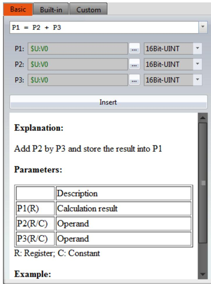
Users can quickly input or select the register and its data type that the user wants to use as parameters; once selected, press **【Insert】** to add the entire statement into the location where the cursor is located in the editor to the right. The usage description and examples of this statement can be checked below the **【Insert】** button.
