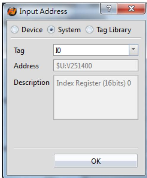
Figure 273 Input Address Dialog-System Tags-Index Register
