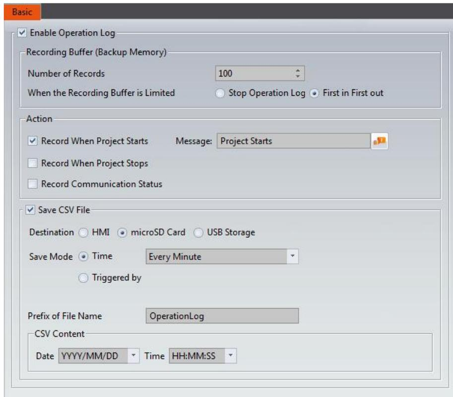
Figure 204 Setting Screen of 【 Operation Log 】
