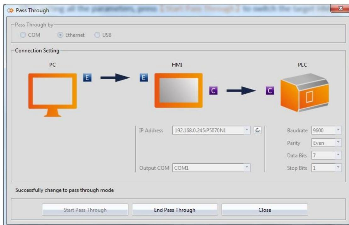
Figure 262 Successfully switched HMI to Pass Through mode
