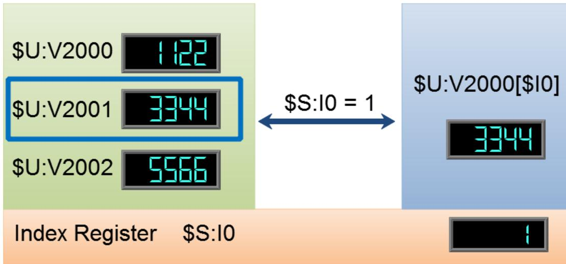
Figure 276 Index Register Example  $\$S:I0 = 1$
