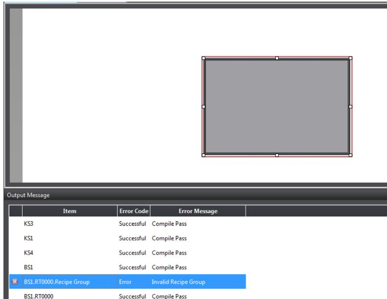
Figure 251 Single click on the compile failure message window to jump to the component
