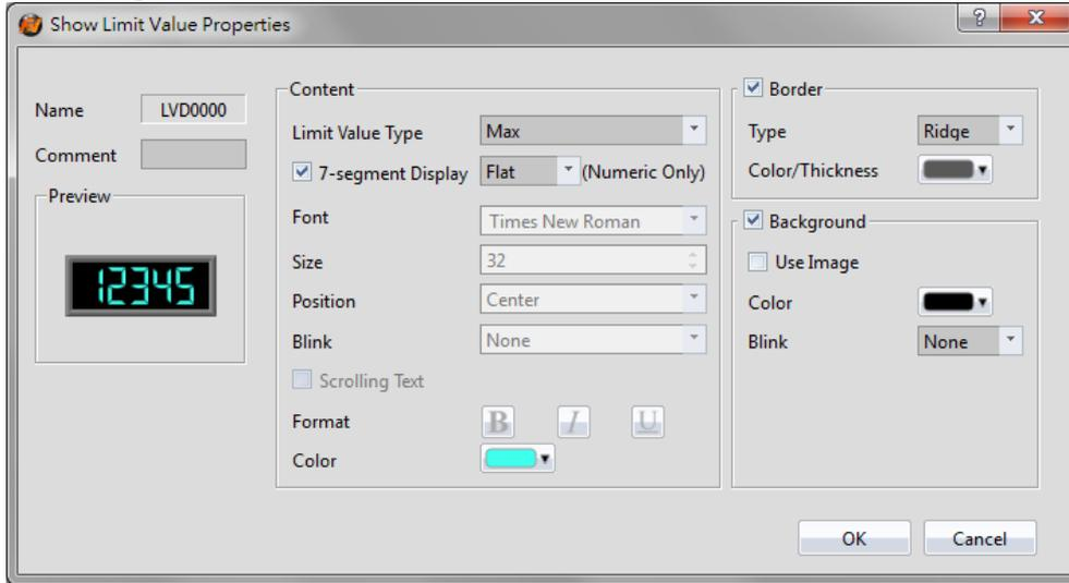
Figure 129 Setting Dialog of **【Limit Value Display】**
