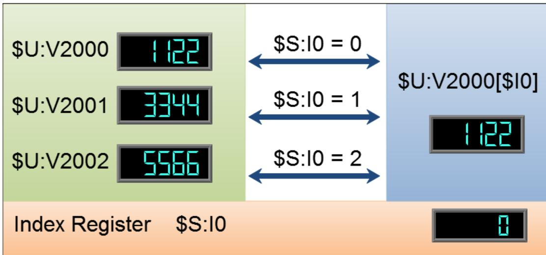
Figure 274 Index Register Example
