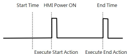
When Power-ON Start/End Action is enabled, if the HMI was turned on outside the Start and End Time interval set for the **【Schedule】** , the HMI will automatically execute the End action once.
