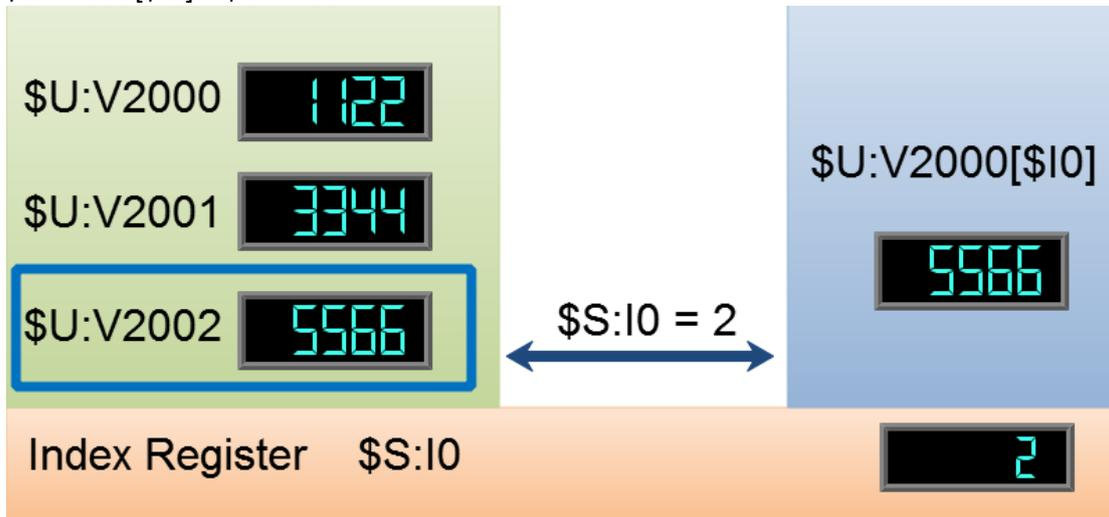
Figure 277 Index Register Example  $\$S:I0 = 2$
