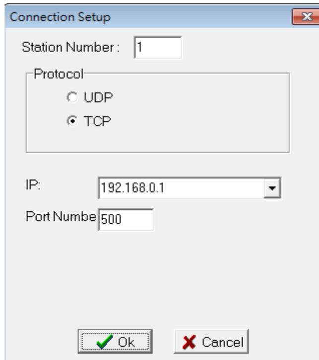
Figure 265 Setting the WinProLadder Ethernet communication parameters
