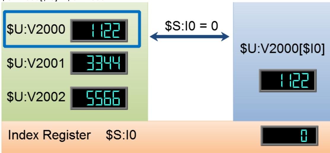
Figure 275 Index Register Example  $\$S:I0 = 0$
