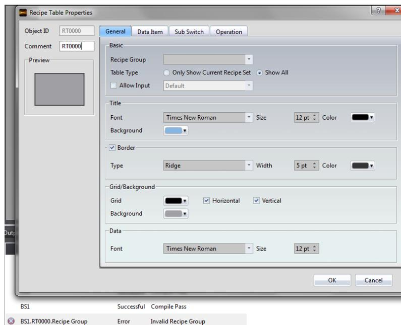
Figure 252 Double click on the compile failure message to open the screen setting
