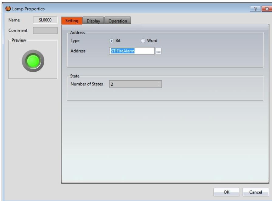
Figure 225 Inputting Address Tag in **【Address Selector】** Edit Field
