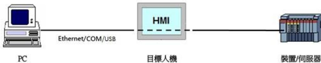
Figure 258 Pass Through architecture
