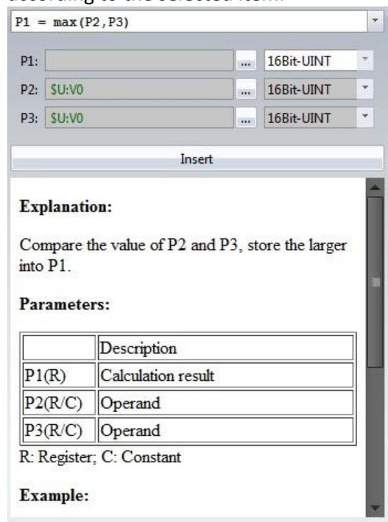
Users can quickly input or select the register and its data type that the user wants to use as parameters; once selected, press **【Insert】** to add the entire statement into the location where the cursor is located in the editor to the right. The usage description and examples of this built-in function can be checked below the
