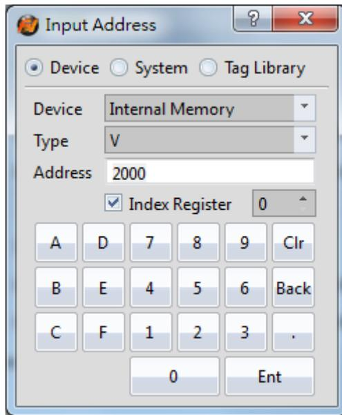
Figure 272 Input Address Dialog-Use Index Register 0
