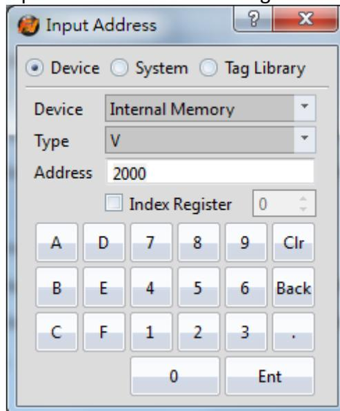
Figure 271 Input Address Dialog-Device Register
