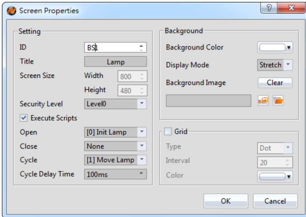
Figure 214 Using Script Setting for the Screen
