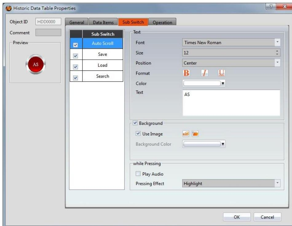
Figure 147 **【 Sub Switch 】** Setting Screen of **【 Historic Data Table 】**
