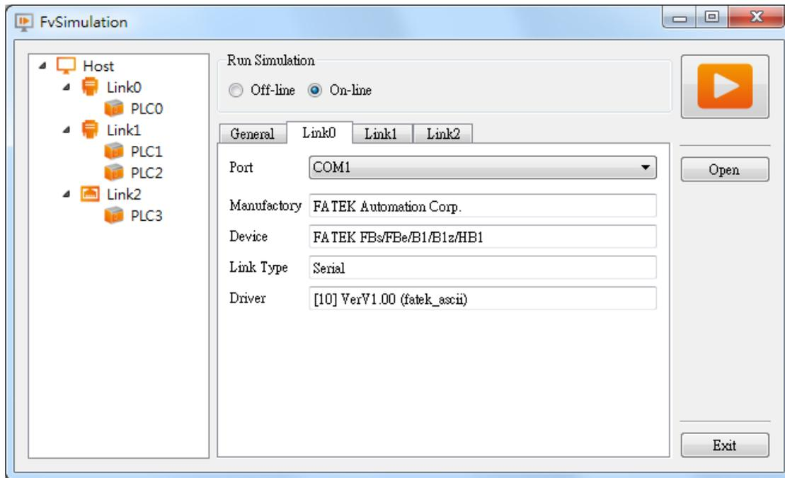
Figure 256 Online simulation connection setting
