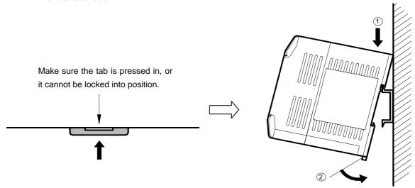
Use a long screwdriver to reach in the hole on the DIN RAIL tab. Pull out the tab to "pulled out" position to remove PLC, as shown in the figure below.
